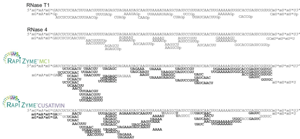
Figure 4. Depiction of identified HPRT sgRNA digestion products for RNase T1, RNase 4, RapiZyme MC1, and RapiZyme Cusativin. Bolded bases signify areas of the sequence where residues were detected in overlapping digestion products. Sequences that end in p (e.g. AACGUUUUp) signifies the presence of linear phosphate product detected in high abundance.
