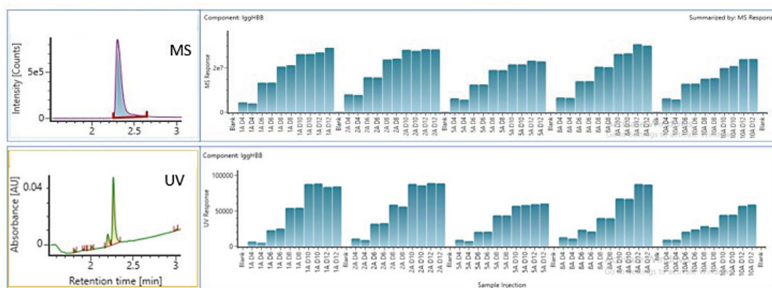
Figure 6. Overlaid bar plot of MS response or UV absorbance across bioreactors and overtime. Each sample was analyzed in duplicate with an overall reproducibility <5%.
