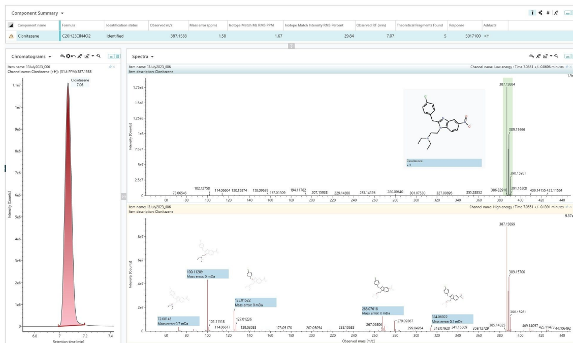
Figure 3. Identification of Clonitazene using waters_connect informatics platform.
