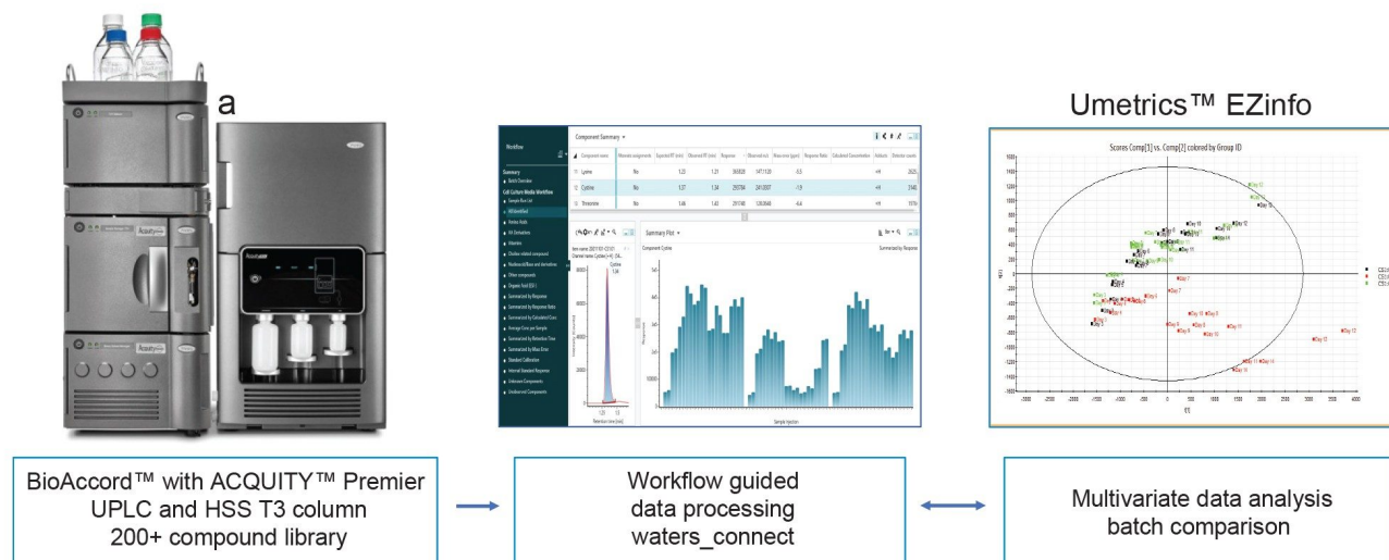
Scheme 1. A schematic illustration of BioAccord System/waters_connect™ based workflow for cell culture media analysis.
