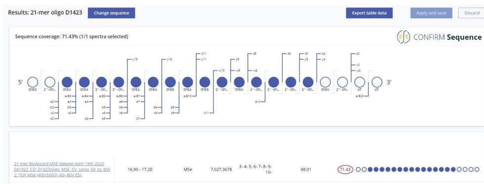
Figure 6. High sequence coverage (> 70%) obtained from high energy MS^E untargeted fragmentation on BioAccord. All precursors of the 21-mer heavily modified oligonucleotide were fragmented using an optimized cone voltage ramp (from 60 to 80 V) applied to the Step Wave of a BioAccord ToF instrument.
