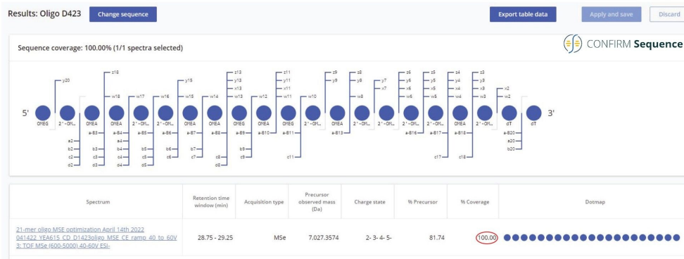
Figure 5. Complete (100%) sequence coverage, presented in a dot-map format, produced by high energy MS E untargeted fragmentation. All precursors of the 21-mer heavily modified oligonucleotide were fragmented using an optimized collision energy ramp (from 40 to 60 V) applied to the collision cell of a Xevo G2-XS instrument.
