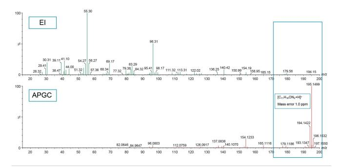
*Figure 3. Comparison of Nylon 6 spectra from EI and APGC highlighting the presence of the protonated molecular ion in APGC.*
