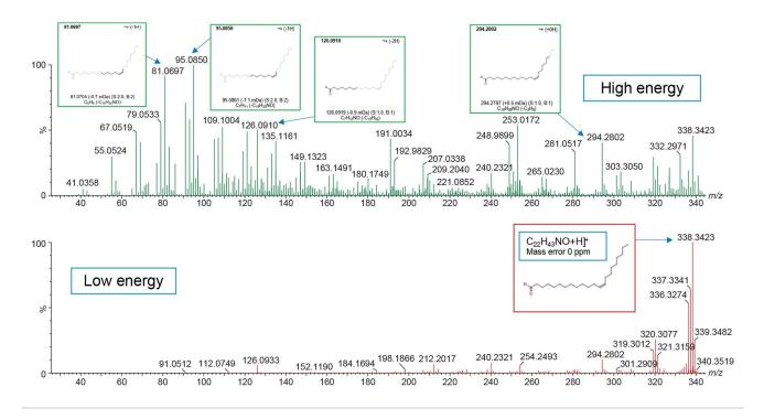
*Figure 6. High and low energy spectra for m/z 338.3423 corresponding to the protonated ion of erucamide using*  $MS^{E}$ . Mass fragments assigned by MassFragment.
