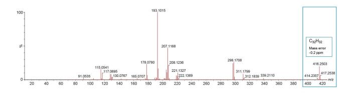
Figure 2. APGC spectrum of the polystyrene tetramer peak eluting at eluting at retention time 22.69 minutes with m/z 416.2503 corresponding to the  $[M]_4^+$  cation ( $C_{32}H_{32}$ ).
