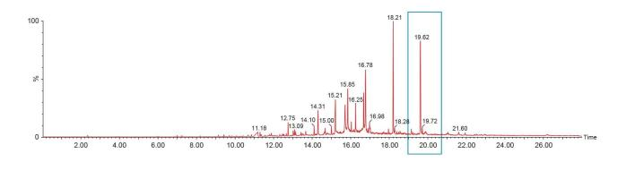
Figure 5. Pyrogram of a biobased plastic bag (Bioplast 500).
