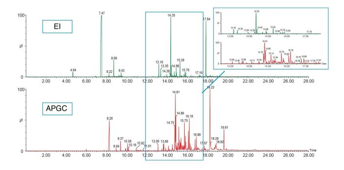
Figure 1. Comparison of total ion pyrograms from El full scan data (in green) to APGC full scan data (in red) for the polystyrene standard.
