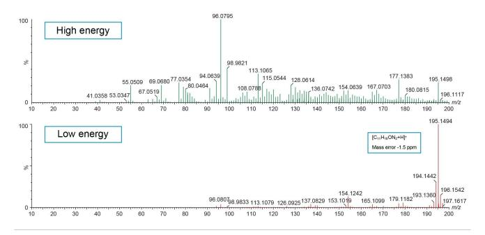
*Figure 4. Example of high and low energy spectra for the protonated ion of N-(5-cyanopentyl)pent-4-enamide using MS<sup>E</sup>.*
