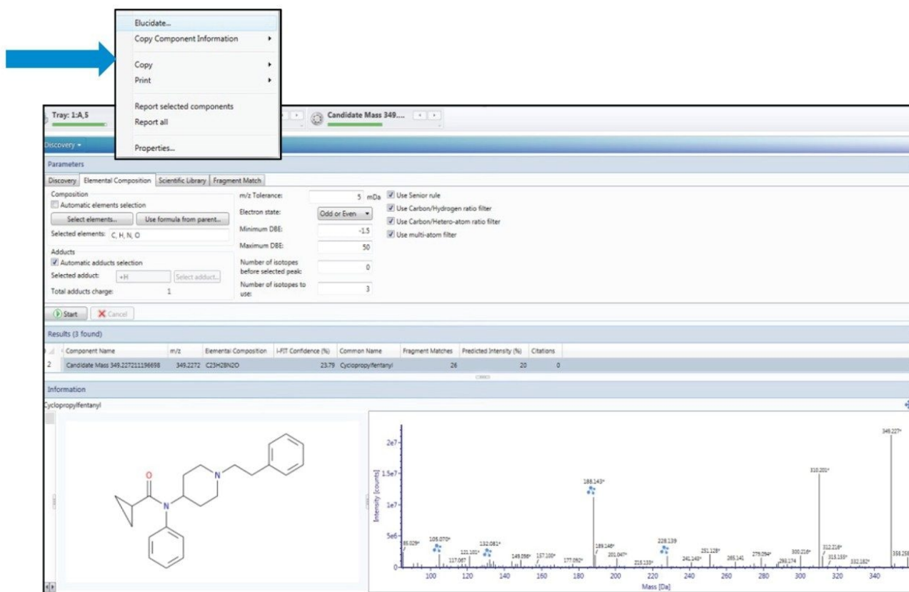
Figure 6. On selection of the component peak of the unknown for the elucidation process, an automated discovery sequence is triggered which includes searching external Scientific libraries e.g., Drugbank, ChEMBL, to provide proposal of likely substances which correspond to the measured accurate mass and matching of theoretical fragments with observed fragment ions. In this example the proposal of cyclopropylfentanyl, based on measured mass m/z 349.2272 together with the isotopic information was supported by 26 matched fragment ions.
