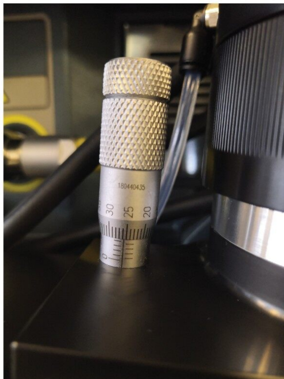
Figure 2. Setting of the vernier scale for the horizontal position of the ESI probe for the analysis of dyes in shrimps. A) position 1 for the analysis of dyes in shrimps B) position 2 for the best signal of leucocrystal violet.
