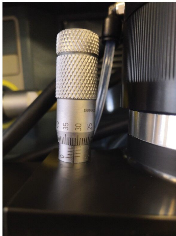
Figure 2. Setting of the vernier scale for the horizontal position of the ESI probe for the analysis of dyes in shrimps. A) position 1 for the analysis of dyes in shrimps B) position 2 for the best signal of leucocrystal violet.
