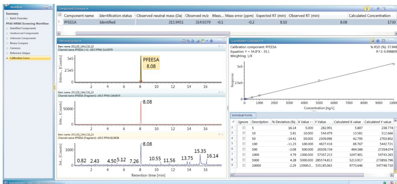
Figure 7. EIC for PFEESA precursor ( m/z 314.9379) and fragments ( m/z 134.9874, m/z 82.9608) PFEESA measured in a lean clay soil extract at 1730 ng/L (8.65 ng/g in the soil). A linear calibration curve over the range (5–10,000 ng/L) is also shown.
