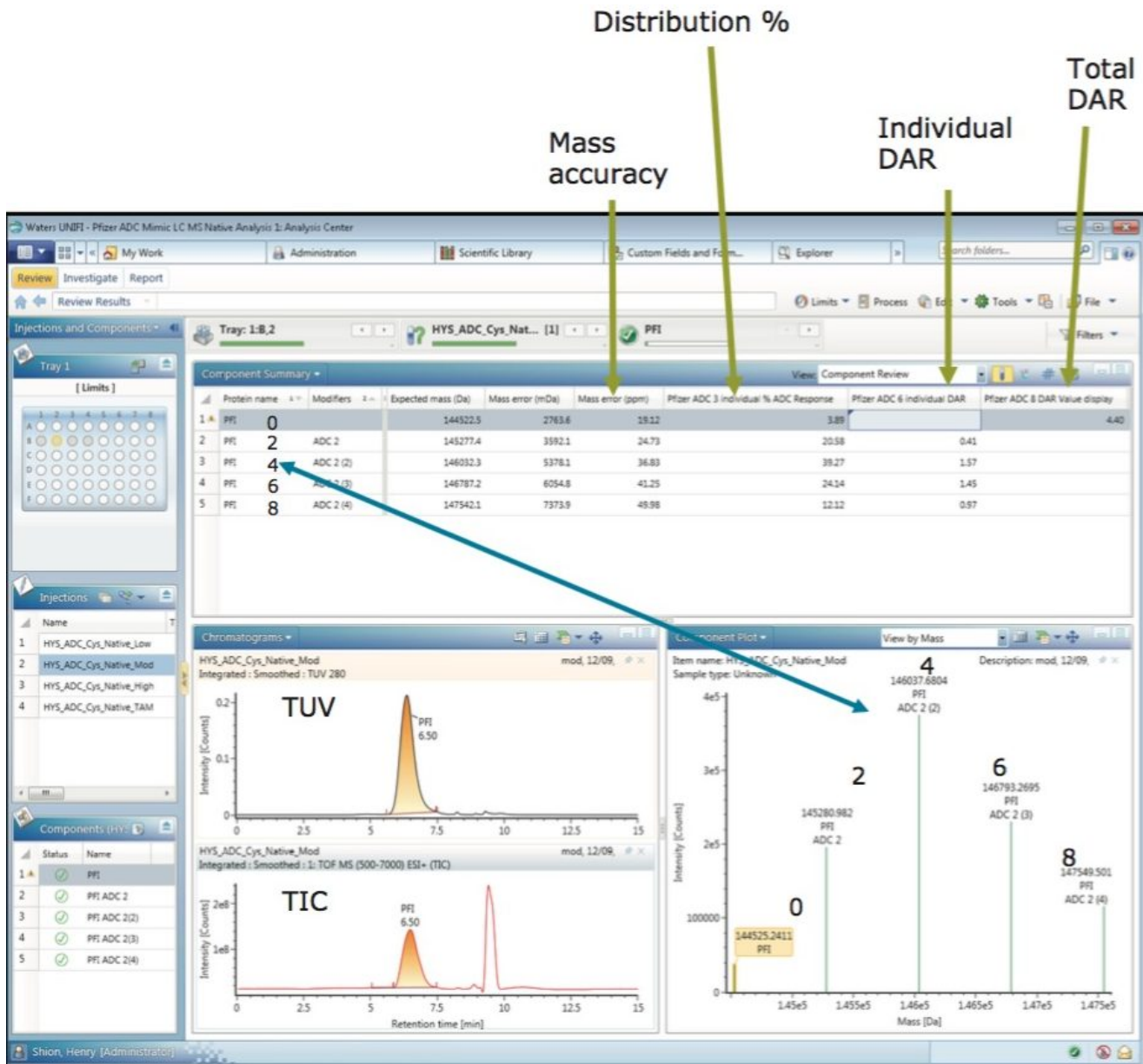
Figure 7. UNIFI review pane shows the automatically process data and calculated DARs from the native SEC-LC-MS experiments.
