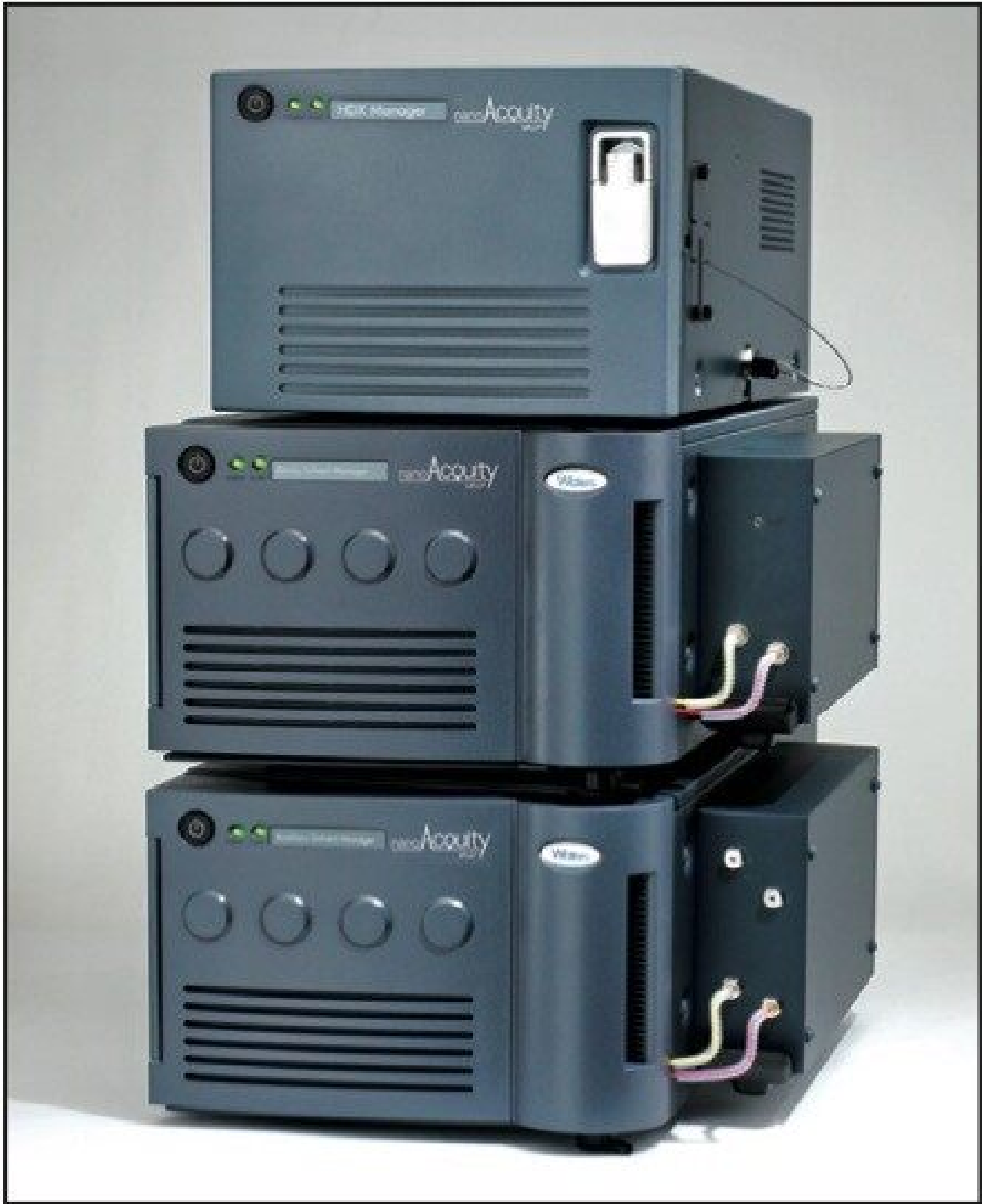
The nanoACQUITY UPLC System with HDX Technology.
